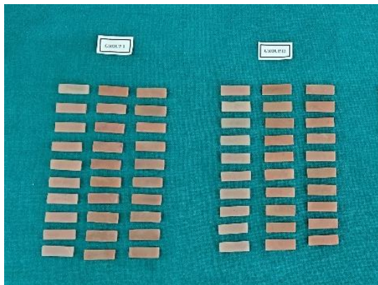
Figure 2: CAD/CAM Pre polymerised PMMA resin and Injection molded PMMA resin layered with gingiva colored composite resin.
